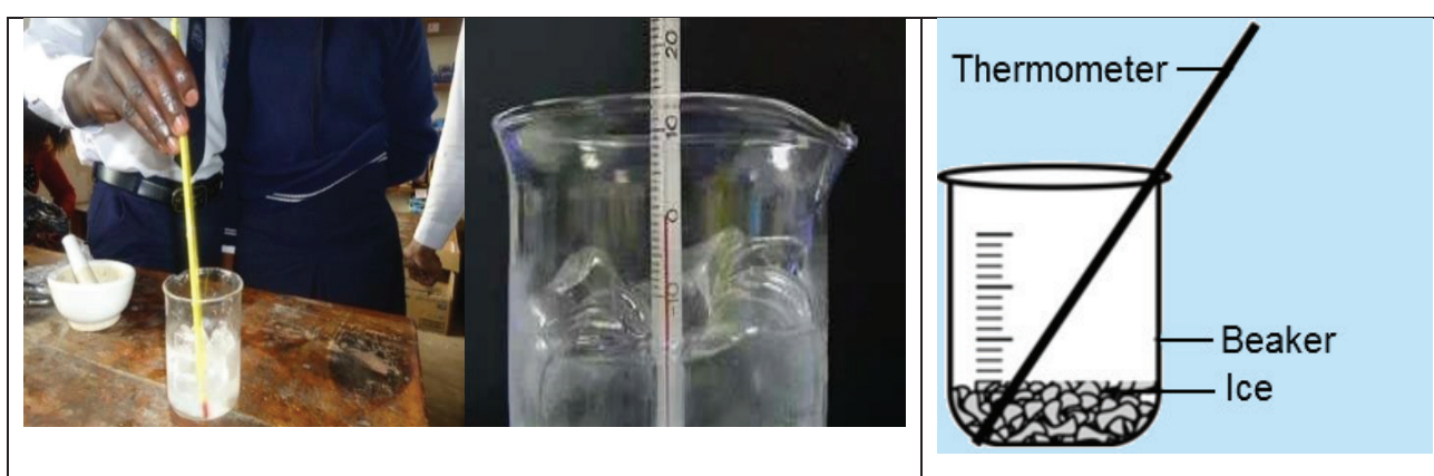
Figure 5.3: Determining the lower fixed point on a thermometer
